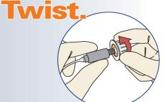
Hold luer access valve in one hand while pushing and twisting the *Swab* Cap in a clockwise direction onto the luer access valve.
