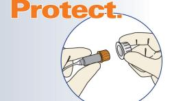
After Swab Cap has been twisted into place, gently pull white plastic holder off luer access valve.
