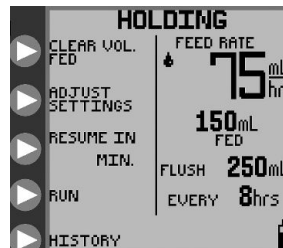
Figure 18A. HOLDING mode options, continuous feeding mode.
