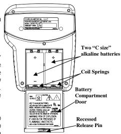
coin into the slot at the bottom of the battery cover and pull in a downward direction. Replace batteries with both positive (+) poles at the top of the battery compartment.
